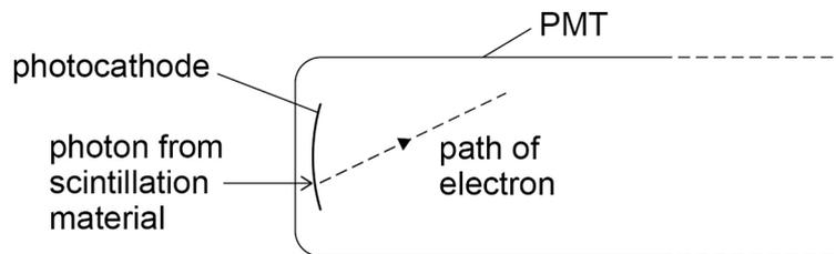
The longest wavelength of light that releases an electron from this photocathode is 630 nm.
