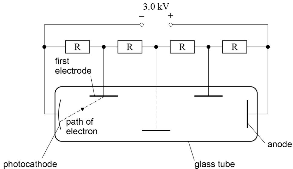
The electrodes, anode and photocathode are connected to a potential divider consisting of four identical resistors  $R$ . The emf of the electrical supply is 3.0 kV.
